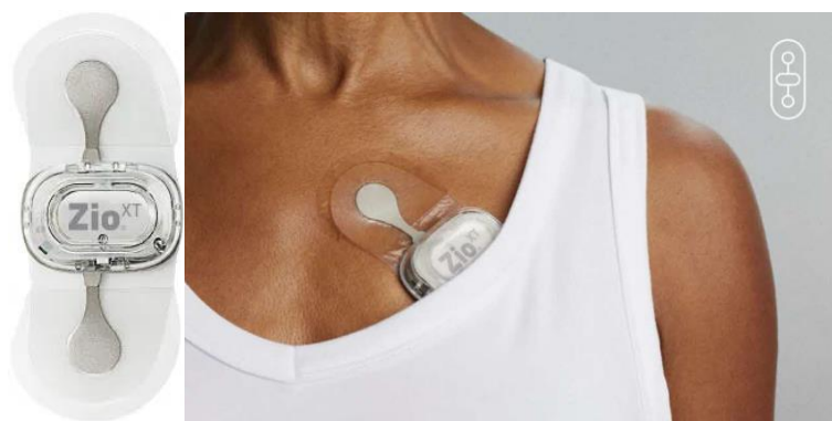
Figure 1: The Zio XT wearable ECG patch (left) and how it is worn by the patient (right). Image adapted from: https://www.irhythmtech.com/providers/zio-service/zio-monitors
